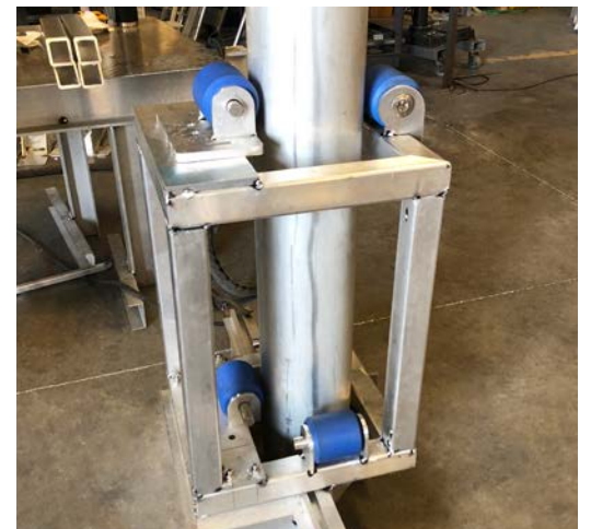
Assembled with 300 Series Stainless Steel Hardware
