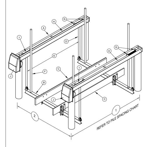
STAINLESS STEEL PILING MOUNT BRACKET, 4 – 3/8" STAINLESS STEEL LAG SCREWS USED TO CONNECT THE BRACKETS TO THE PILING AND 2 – 3/8" CARRIAGE BOLTS USED TO CONNECT THE BRACKETS TO THE LIFT CHANNELS
