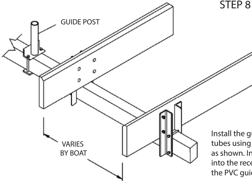
Install the guide pole receiver tubes using bolts and backer plates as shown. Insert the metal pole into the receiver and cover with the PVC guide pole.
