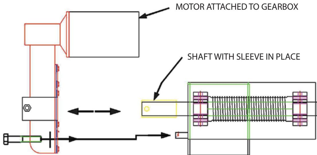
ATTACH TORQUE BOLT THROUGH THE GEARBOX EAR AND THROUGH THE TORQUE NIPPLE. REPLACE THE COVER.
