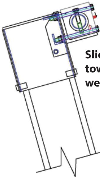
**Slide the drive head over the beam winder facing toward the water. Drill two 7/16" holes through web of I-beam and fasten with 3 1/2" bolts provided.**
