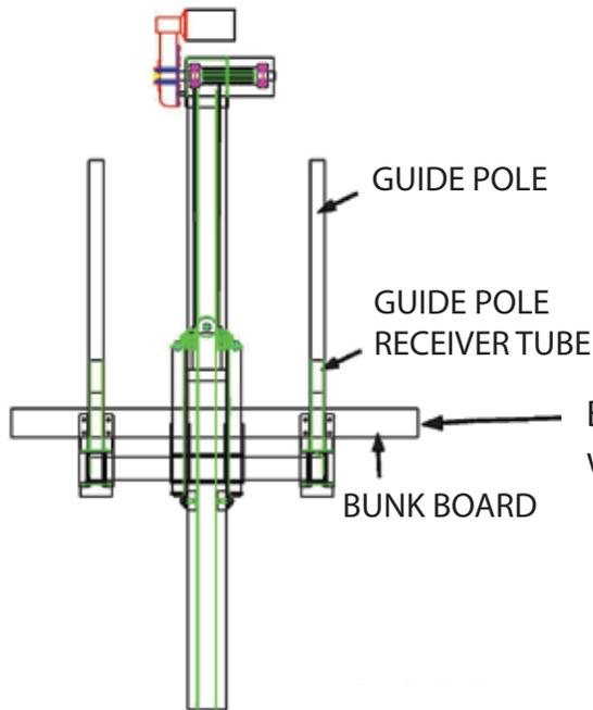
Bolt the bunk boards to the brackets with the bolts provided.
