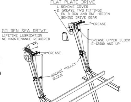
Golden Boat Lifts are designed to provide years of service with very little maintenance. We recommend grease in the points depicted two times per year. The Sea-Drive is lubricated for life. Flat Plate - recommended to grease very often (every 10 uses).
