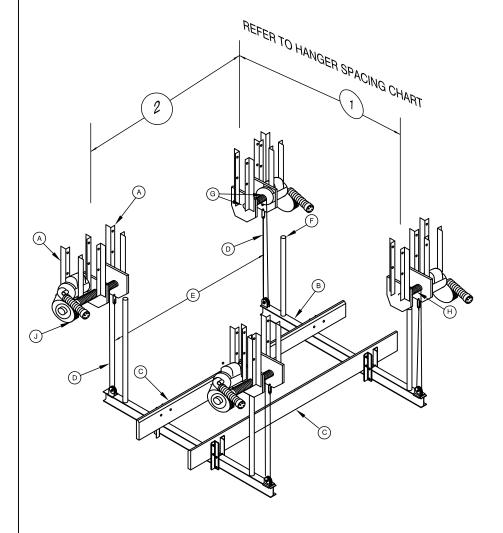
6061-T6 ALUMINUM HANGER MOUNT BRACKETS-RECOMMENDED ATTACHMENT BASED ON BRACKET CONFIGURATION. VERIFY ADEQUACY BASED ON ACTUAL SITE CONDITIONS:
