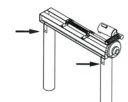
6 LOOSELY ATTACH GUIDE POLE BASES. THEY WILL BE ADJUSTED LATER.
