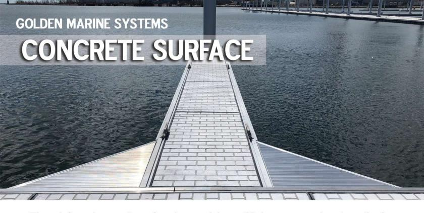
The reinforced concrete surface has a minimum 28 day compression strength of 5,000 PSI, per ASTM standard C-94. The walking deck is poured in one monolithic pour over a galvanized welded wire reinforcement that meets ASTM standard A-185.
