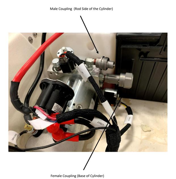
**Leaks:** Unit should be free of leaks, However please tighten and fittings if you notice a leak.
