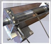
**Box Construction for Drive Connection to Track Beam**
