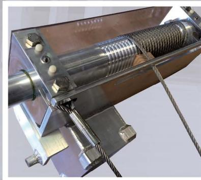
Box Construction for Drive Connection to Track Beam
